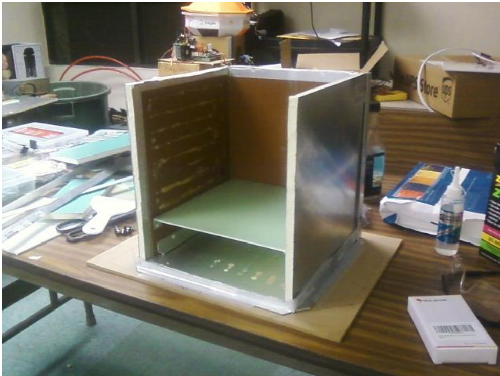
Figure 1 Three walls, base flanges, and test bay floor together on mounting-plate-copy for fit check. Looking in through the starboard wall, which is not present in the photo.
