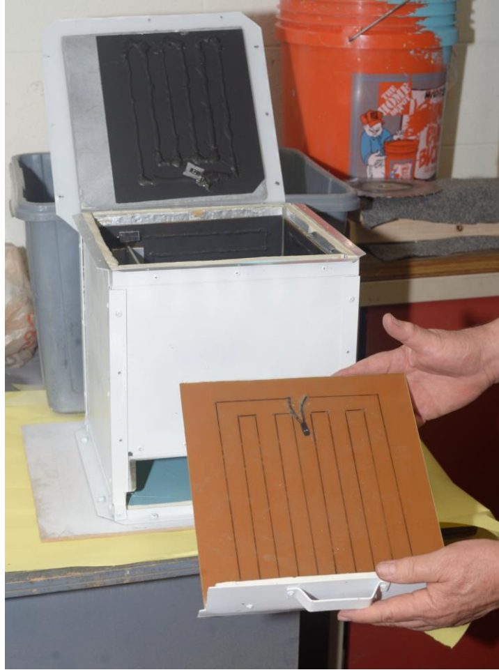
Figure 2: The UB Testbed container opened and with the Electronics Bay drawer puller out. Nichrome wire patterns are visible on the walls.
