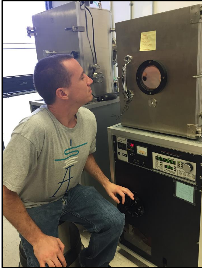
Fig. 2 Chris is working on deposition of thin film using a high vacuum system.
