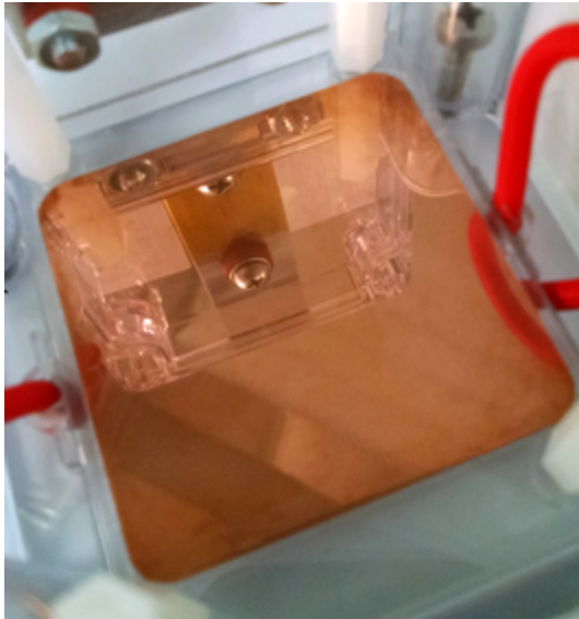
Left: Copper plate inside the EPC assembly after flight Right: Copper plate placed inside a casting mold for acrylic epoxy embedding.
