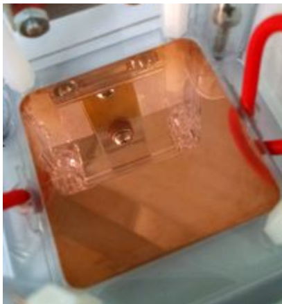
Left: Copper plate inside the EPC assembly after flight Right: Copper plate placed inside a casting mold for acrylic epoxy embedding.
