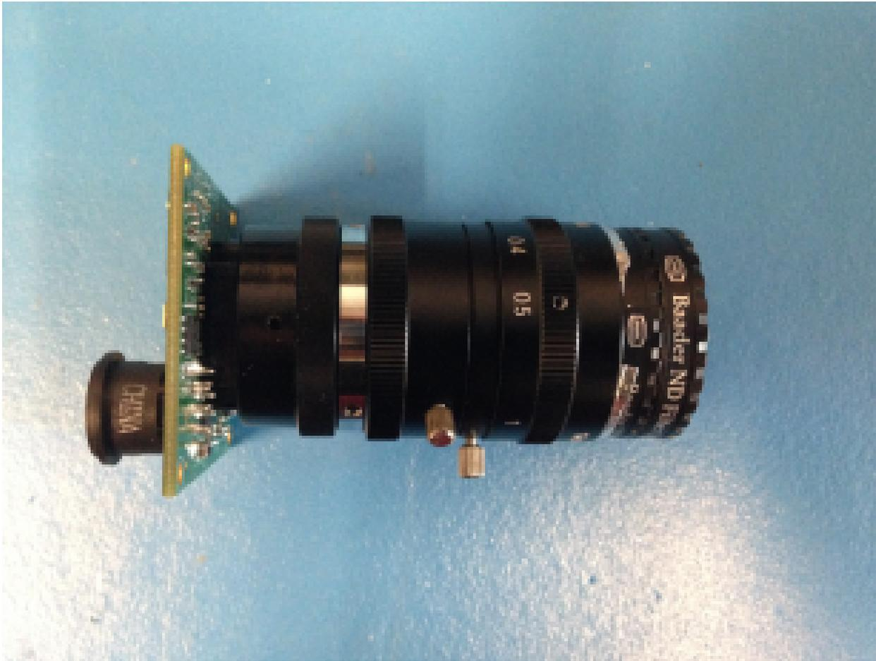
Figure 2: ADCS Camera equipped with two neutral density filters
