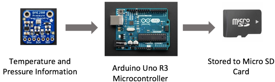
Figure 6. Information from the BME280 Temperature/Pressure sensors will be sent to the Arduino and subsequently stored to the onboard micro SD chip.
