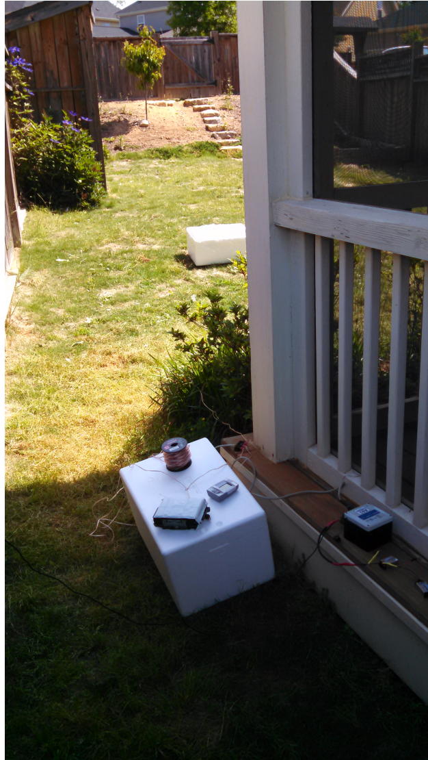
Figure 1: Microphone at approximately 70 C in a solar oven (background) and microphone at approximately 10 C in a cooler (foreground) with a microphone at ambient temperature and the data logging system.
