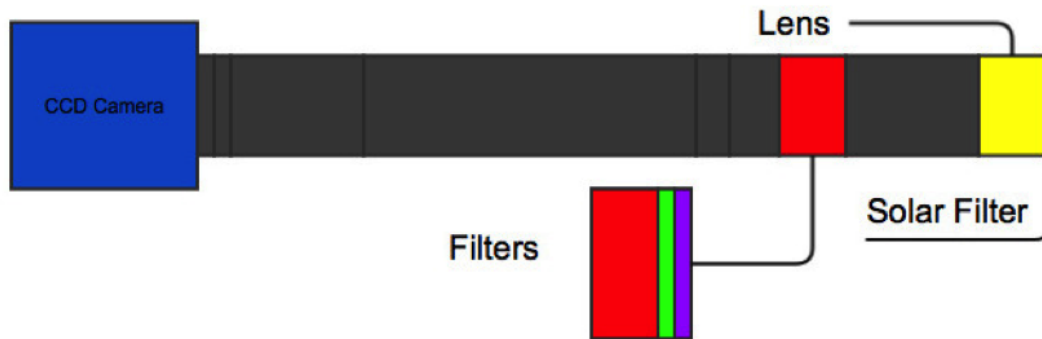
Figure 3: Science Camera System fully equipped with a solar filter, IR filter, UV filter, and H-alpha filter.
