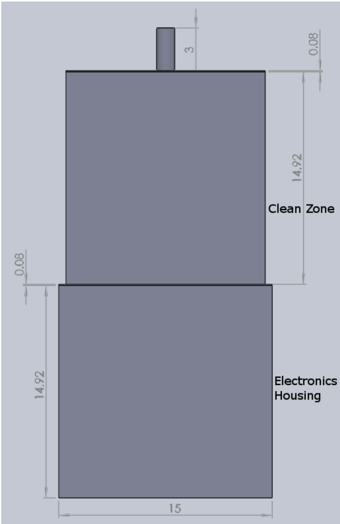
Figure 2: Side View of SIMBA with both sections labeled (all units are in cm)
