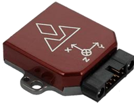
Figure 9. The VectorNav VN-100 Rugged IMU. The VN-100 measures 3.6 cm x 3.3 cm x 0.9 cm.
