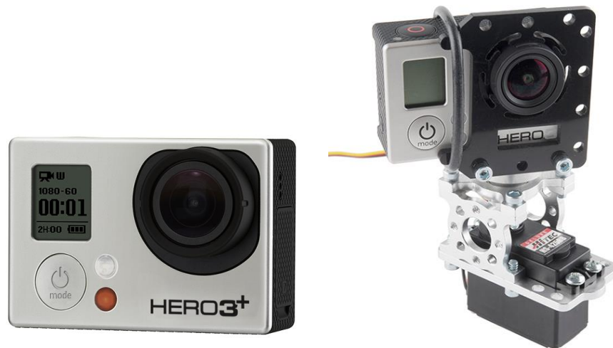
Figure 13. (Left) The GoPro HERO3+ WiFi-enabled camera for the video downlinking system. (Right) The servo mount for the GoPro. The GoPro measures 5.9 cm x 4.1 cm x 2.8 cm.
