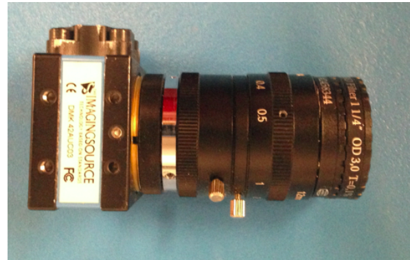
Figure 2: Photo of the ADCS Camera that flew; the neutral density filters are stacked on the right end
