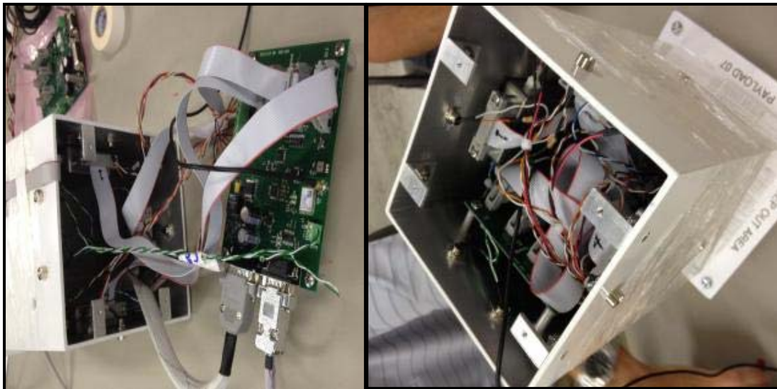
Fig. 11 (b) Inregration of sensors boxes, payload and PCB and Top view of payload
