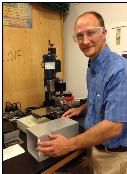
Fig.8 (l) Ken (UNF) fabricating the payload body using CNC machine (Micromill 2000)
