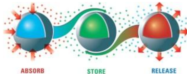
Figure 3 – Reaction of the PCM's absorbing, storing and releasing energy
