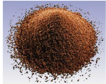
Figure 9 – Encapsulate RubiTherm GR at 42°C
