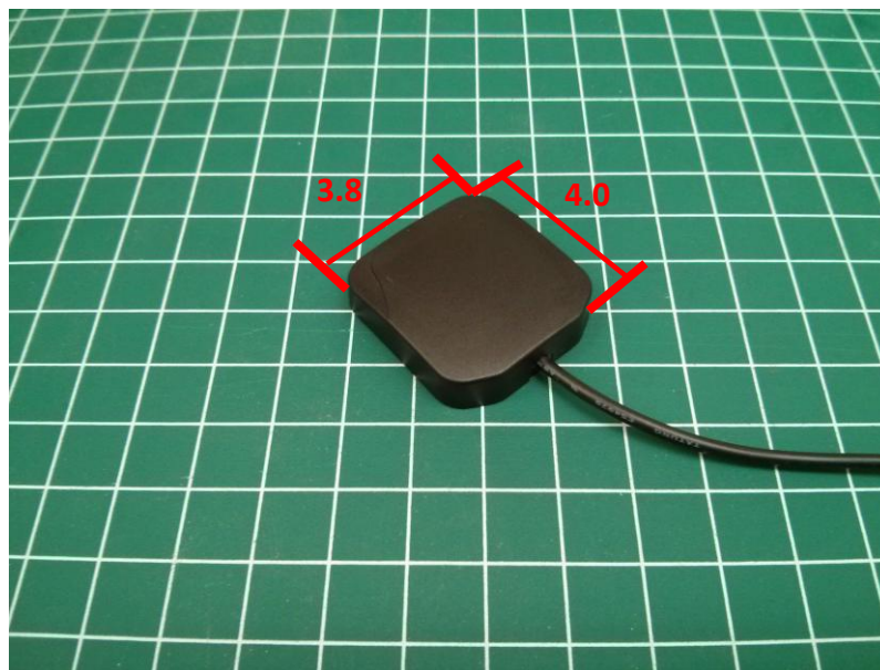
Figure A15. New GNSS antenna with dimensions in centimeters. The antenna is capable of receiving both GPS and GLONASS signals, and is in a protective housing.
