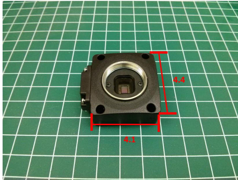
Figure A16. Point Grey Research Chameleon camera with dimensions in centimeters.
