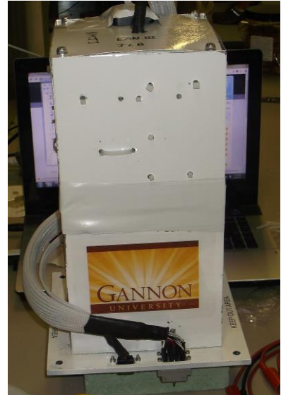
Figure 2. Completed, sealed GU-HARD-PL03
