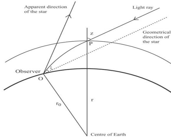
**Figure 1. An example of how signals are affected by refraction (Hohenkerk, C. Y. & Sinclair, A. T. 1985)**
