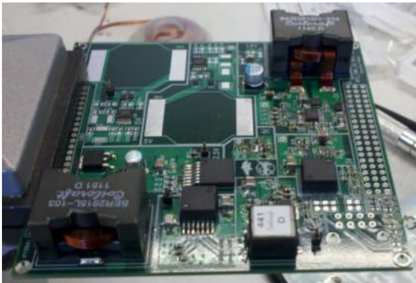
Figure 1: Power CCA during assembly and test.
