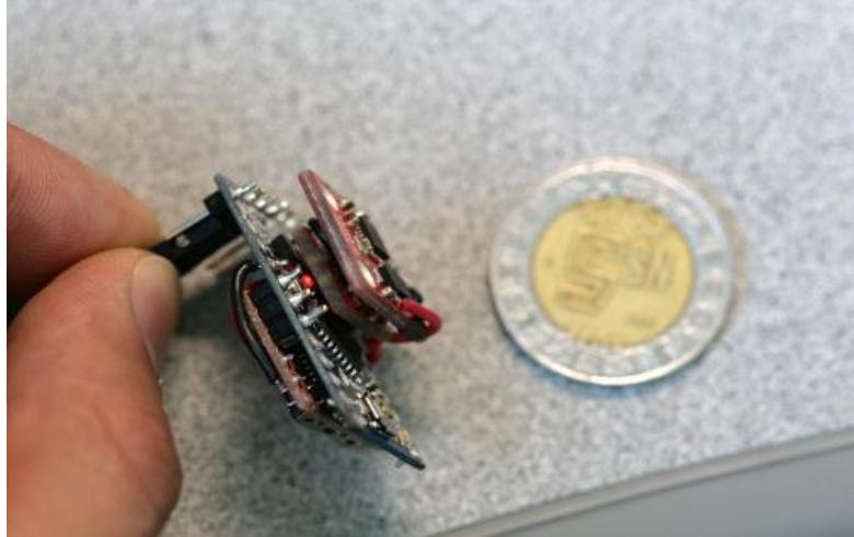
Figure 2: Photograph showing the prototype for the EFM control and data collection system. Coin is about the size of a quarter.
