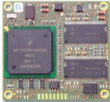
Figure 6. Flight computer (32-bit PowerPC Phytec MPC5200B-tiny SoM [11]).
