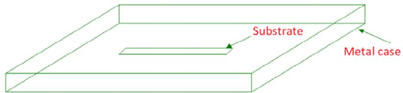
Figure 5. Schematic diagram of housing for substrate (overall size: approximately 3 x 4 x 1 cm)
