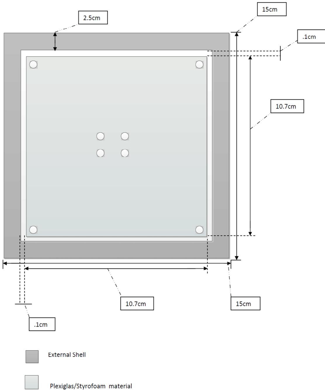
Figure 6. Top view of the proposed payload
