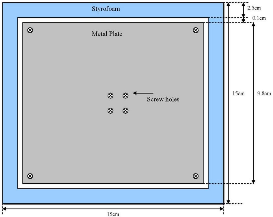
A metal plate will be placed at the bottom of the box and screws holes will go through both the metal plate and the Styrofoam to ensure a secure attachment to the rest of the payload
