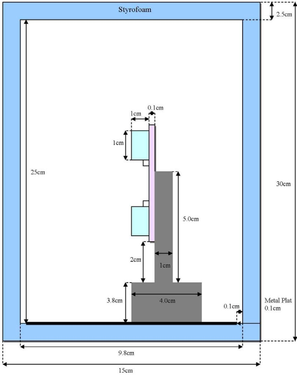
Figure 9. Side cut view of payload
