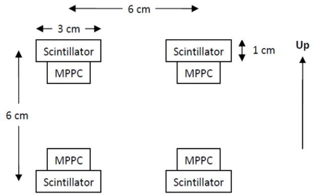
Figure 2. Detector Module - scintillator layout
