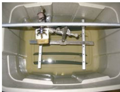
Figure 5: Picture of a student constructed tank and holders used to develop the film (Fontenot et al. 2007, Fig. 5)
