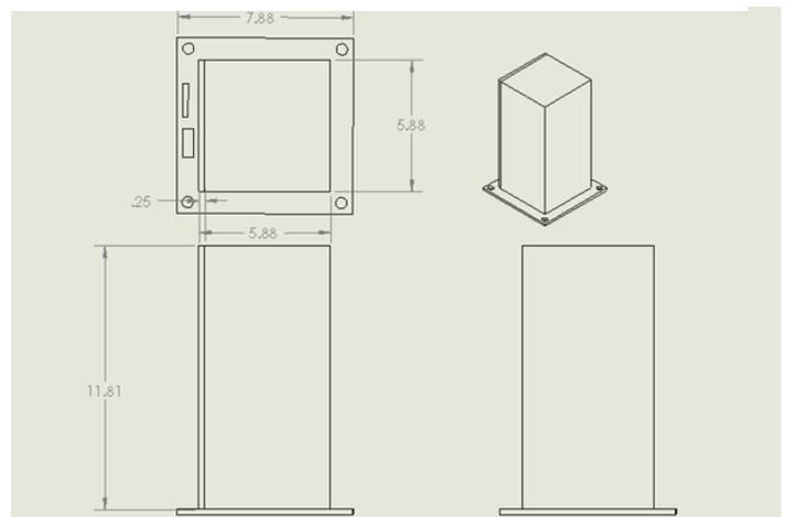
Figure 6 – Fully Assembled Payload Mounted (inches)
