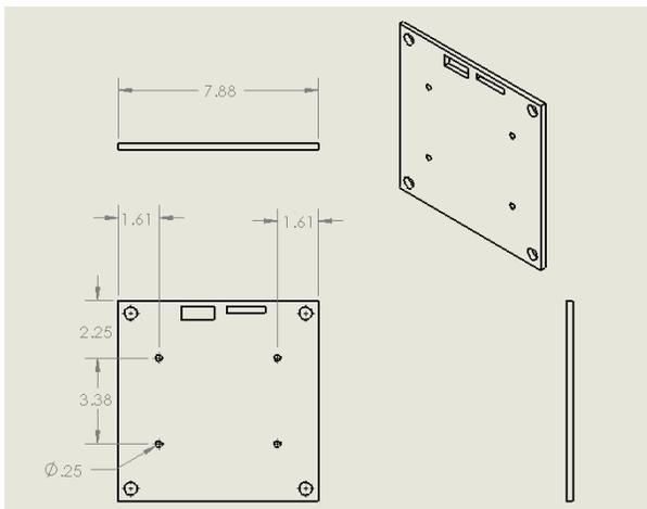
Figure 5 - Payload Mounting Plate Modifications (inches)
