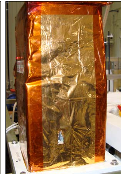
Fig.8c Thermal blanket (golden color) on Payload body
