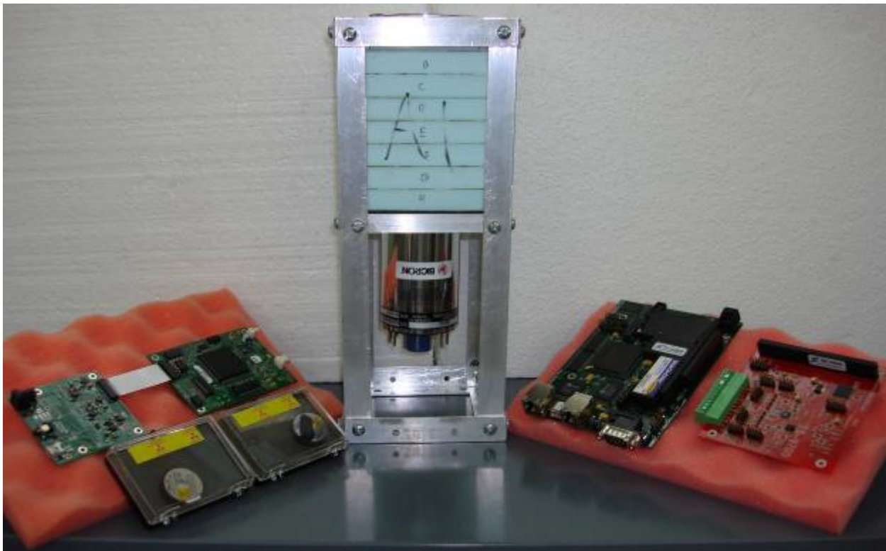
Figure 2 (From Left to Right): PC4-2, DP4, Scintillation Detector Contained within the Structural Frame, TS-5400, TS-9700, shown with two radiation test sources on the left
