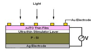
Chemically cleaned p-type silicon wafer will be used as a base of solar cell, while n-type indium tin oxide (ITO) thin film used as a window. 5000 Å thick Ag film electrode will
