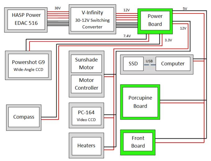
The four power and four ground lines from the EDAC 516 connector are routed through a 12V switching converter. The resulting 12V line is run through 3.3V, 5V and 7.4V converters. Using these three outputs and the original 12V line, every subsystem within the payload has the necessary voltage.
