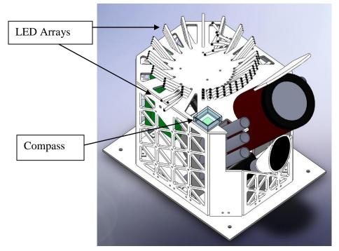
On the top of the external structure, there are 108 LED photometers. One array is a 360° and another is a multi-angle array that faces the same direction. A digital compass is also included and mounted to the roof.
