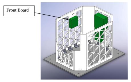
The front board will be mounted directly to the left wall of the payload.
