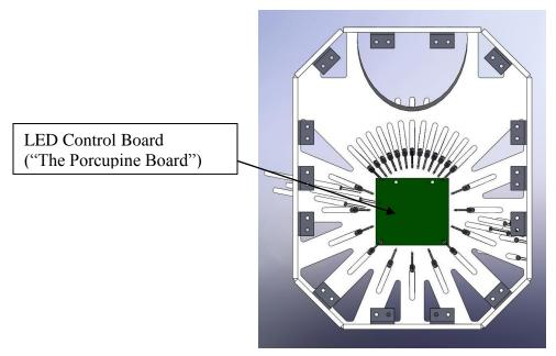
Mounted to the roof, in the middle of the 360° LED array, is a board that primarily controls the data obtained from the LED photometers.
