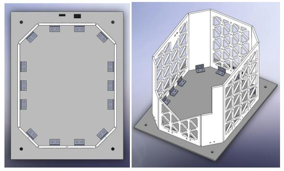
The payload's walls will be attached to the PVC mounting plate using 14 right angle brackets as shown. The fasteners that will be used are 10-32 socket-cap bolts and nuts.
