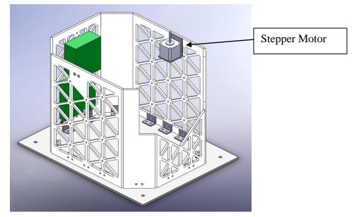
The stepper motor will be attached to a universal joint that is connected to another universal joint via an extension rod and it will control a sunshade that is attached to the telescope.
