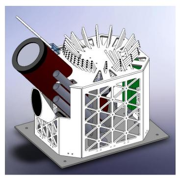
The image above shows an isometric view of the BOWSER payload. On the next page is a drawing that shows external measurements of the payload. Earlier in the year, Team BOWSER confirmed that the protrusions will be allowed for the flight.
