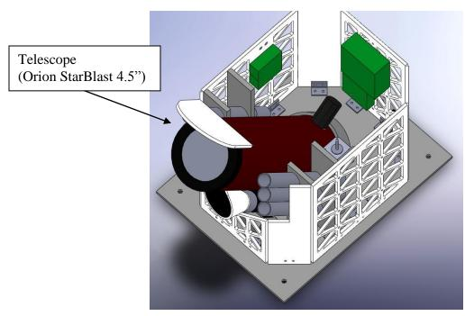
The telescope that we are using is a modified Orion StarBlast 4.5" Newtonian telescope. A sunshade will be attached to the top of the telescope as shown in case the telescope faces direct sunlight.
