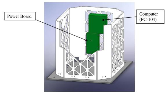
The power board is mounted directly to the back wall. The computer attaches to a thin steel plate that will attach to the back wall as well.
