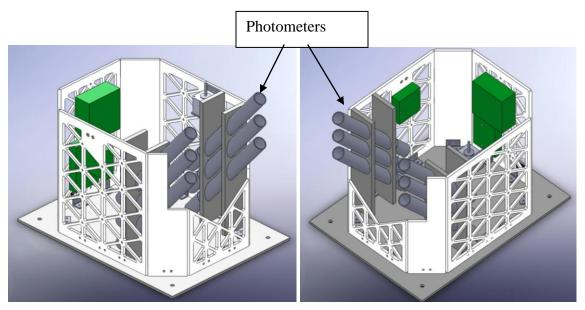
The photometers are used to gather light-sensing data that is required for our mission. They are mounted to the left and right walls.
