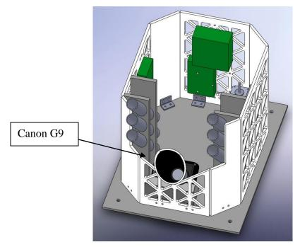
The Canon G9 is Team BOWSERs chosen wide-angle imaging device. It is mounted on its own ramp and a baffle for stray light is included.
