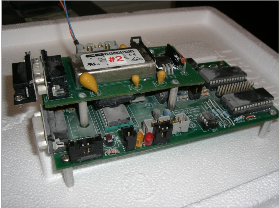
Figure 36. Conformal-Coated Circuit Board and Power Supply for Flight
