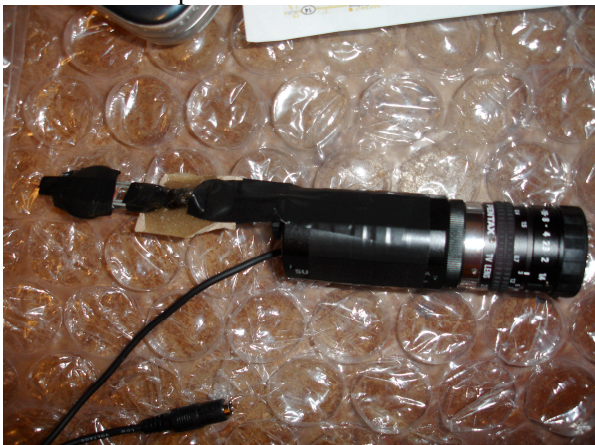
Fig. 6: CCD Camera system similar to what will be present onboard the DIE HARD payload.
