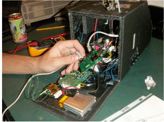
Fig. 3: The internal components for a stabilization and CCD camera imaging system.
