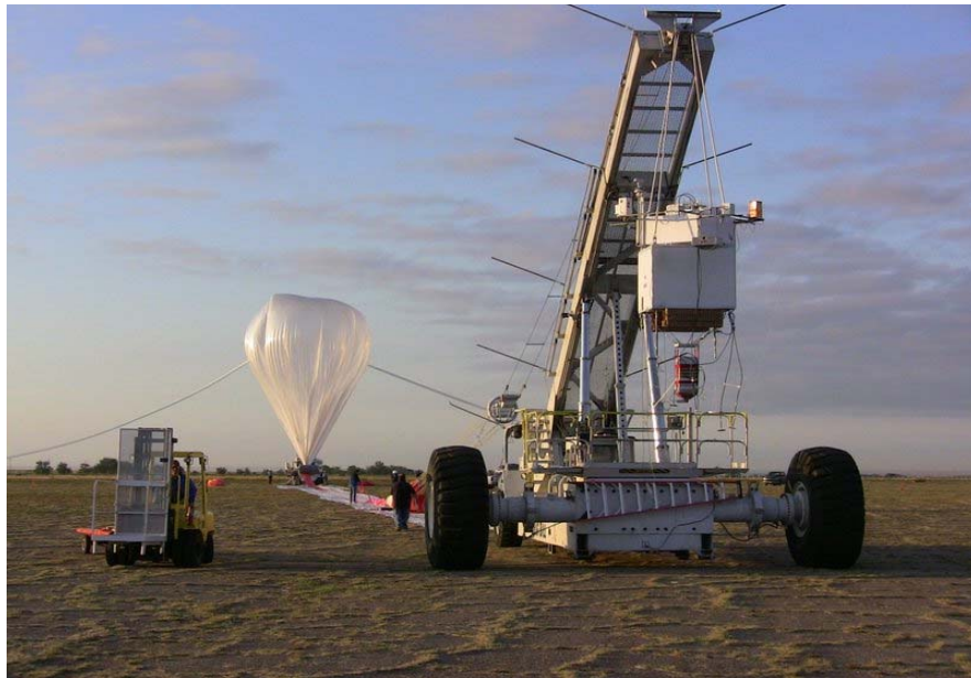
Fig. 16 Balloon attached with parachutes and HASP payloads (Courtesy: HASP)
