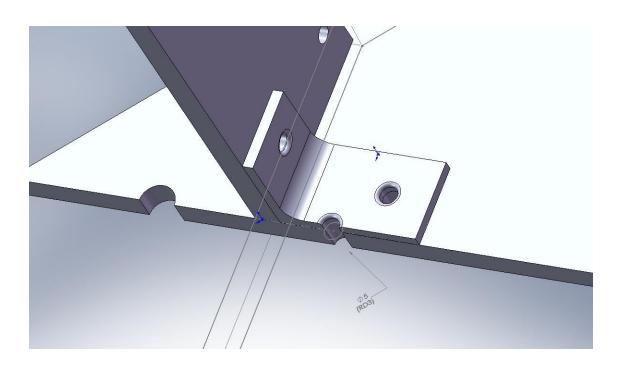
This is a cross sectional example of how we're going to be mounting our primary structure to the mounting plate. The way we're going to attach the structure is by using an L bracket that attaches to the walls and the primary mounting plate along the bottom of all the exterior walls. This bracket will bolt through both the walls and the mounting plate itself with washers on the under side of the mounting plate to distribute the force from the structure.
