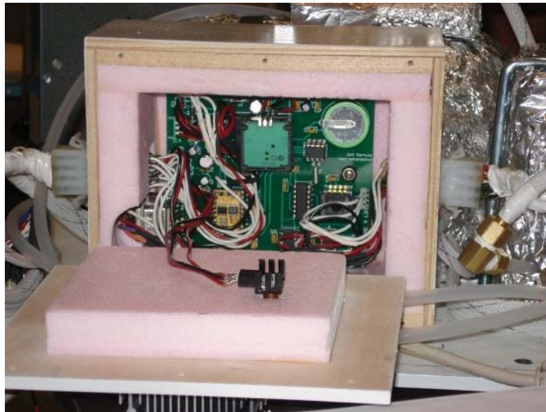
Figure 10: A view of the circuit board after being securely mounted in the insulated housing
