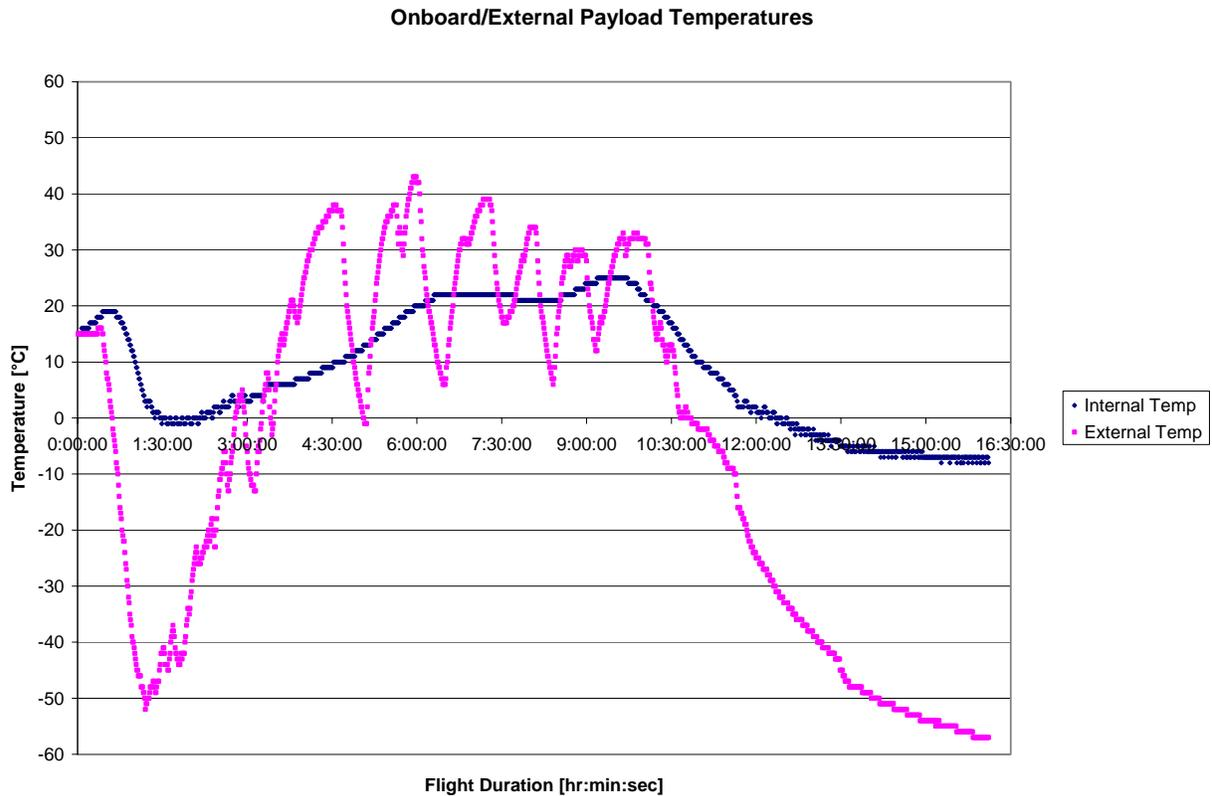
**Figure 6. Internal and external temperatures for TIBE payload.**
