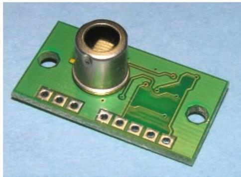
**Figure 3. Devantech 8x1 thermopile array.**
