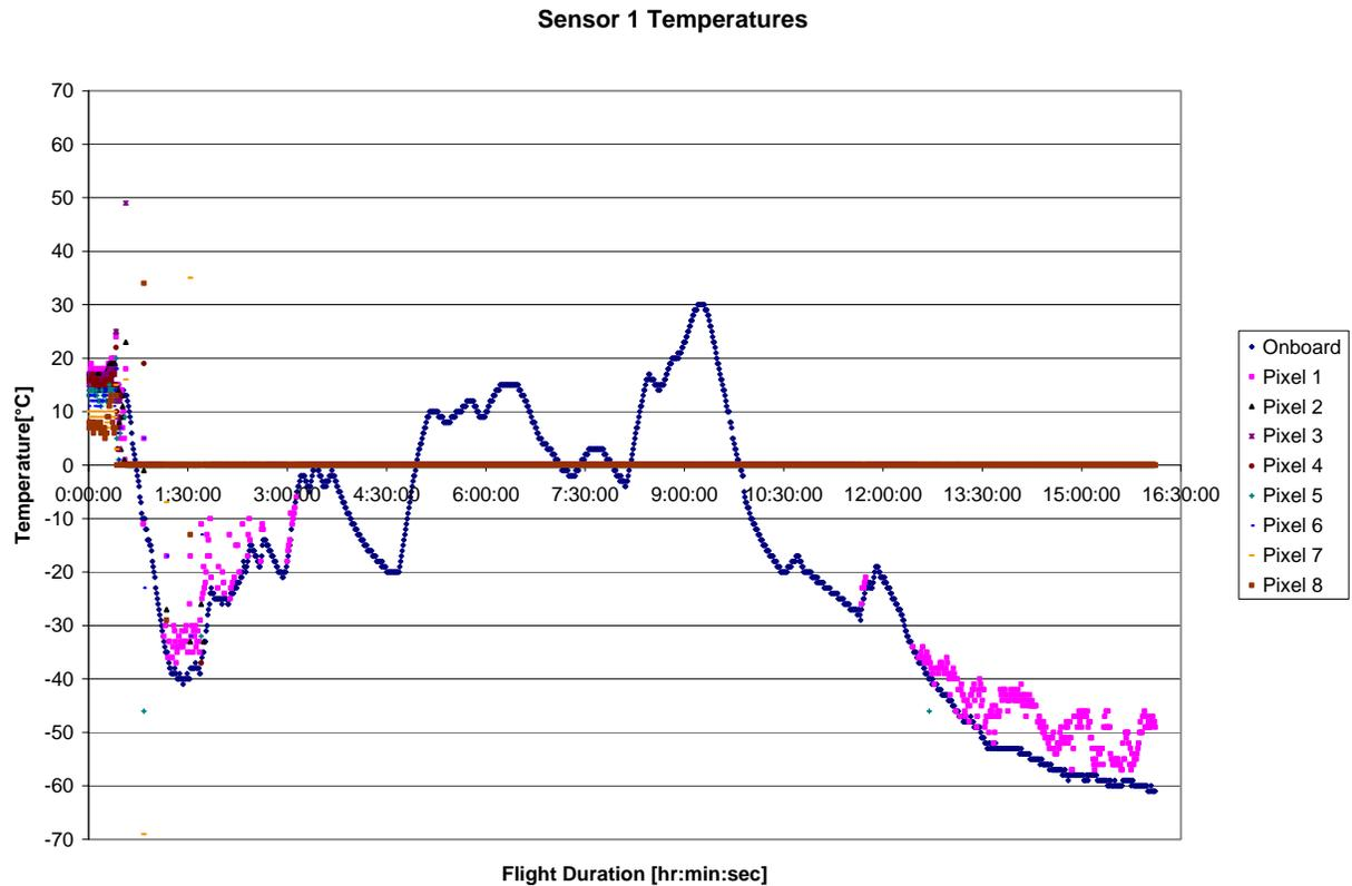
**Figure 7. Sensor 1 (0° arc position) temperature data.**
