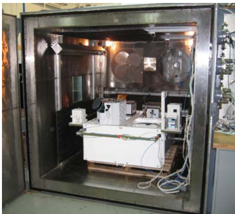
Figure 8: HASP and student payloads in the CSBF BEMCO chamber in preparation for thermal / vacuum testing.
