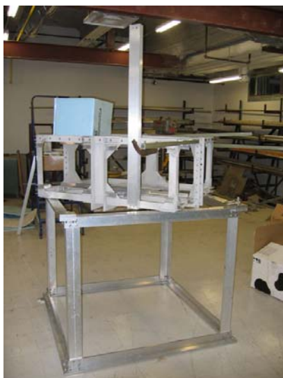
Figure 2: HASP structural framing
